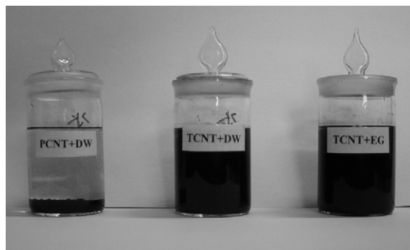
Fig. 2. Stability comparison of nanofluids containing PCNTs or TCNTs.
